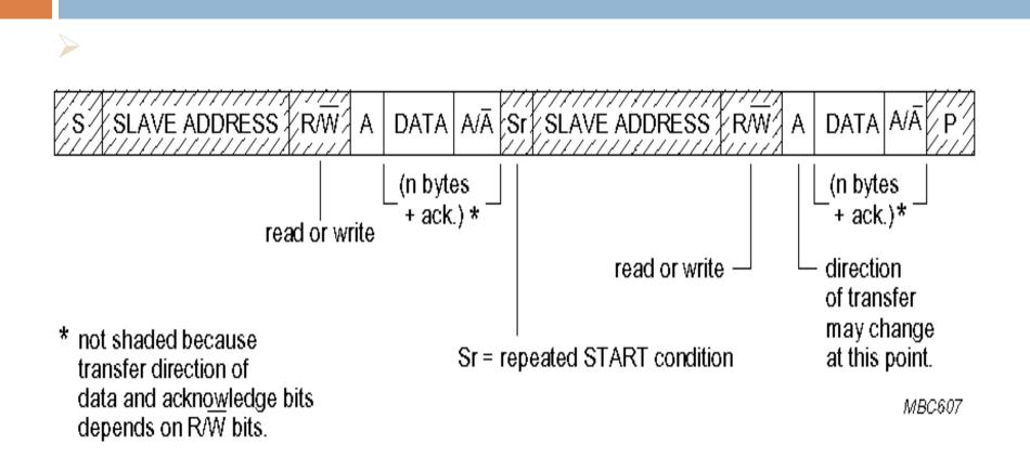
A repeated start avoids releasing the bus and therefore prevents another master from taking over the bus
