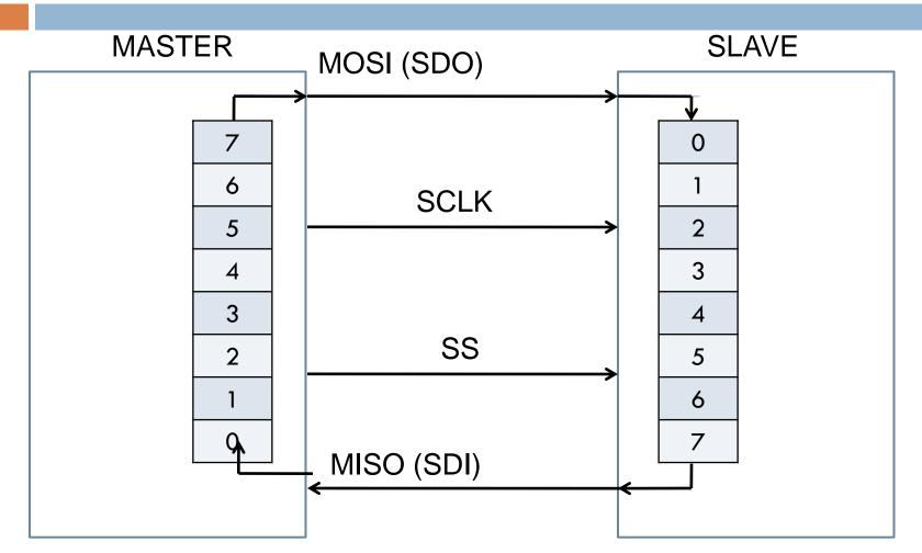
The registers within the master and slave act like shift registers shifting one bit on every cycle of the SCLK.
